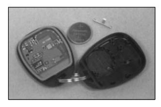
To replace the battery in the transmitter:
